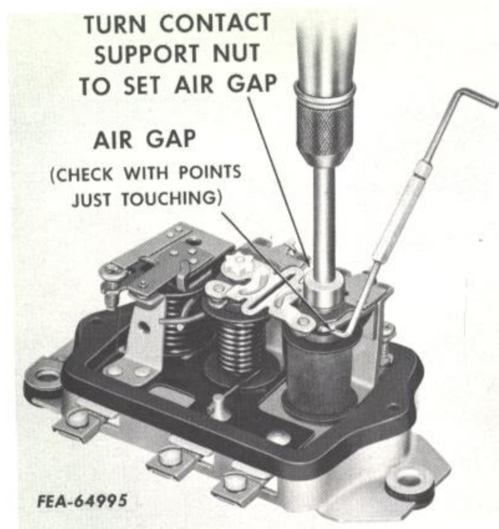
Illust. 38. Voltage regulator air gap check and adjustment (3-unit regulator).
