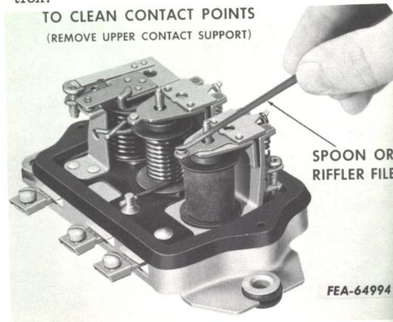
Illust. 28. Riffler file used to clean flat contact points in regulator (3-unit regulator shown).
